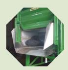
Wide discharge opening for higher transfer rate, prevent clogging or long waiting time
